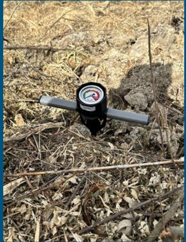
Ripped area- decompacted
