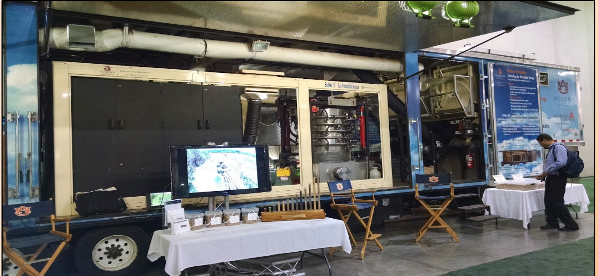
Auburn University's mobile biomass gasifier.
