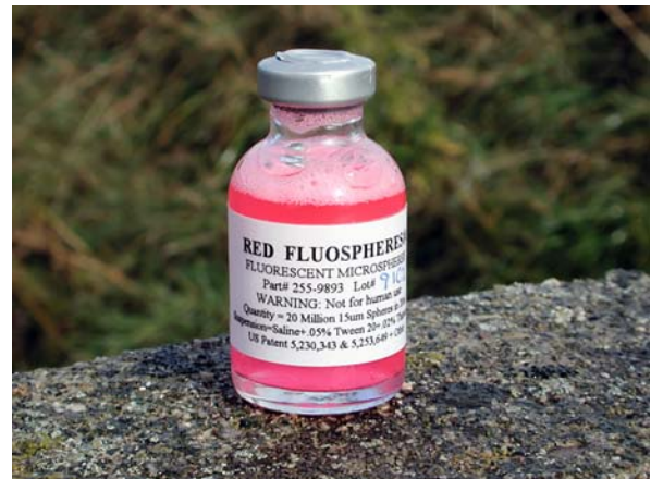
Figure 3. Bottle of 15 \mu\text{m} microspheres used as a tracer for mine water investigations.
