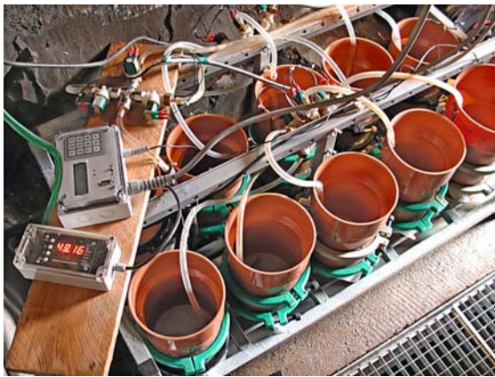
Figure 2. Sampling equipment (Multiple Filter Storage Tool: MeFiSTo) for a multi-tracer test with microspheres including flow-meter and electronic control device.
