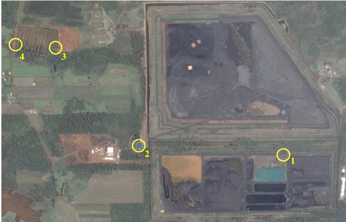
Figure 2. Locations of sample collection stations 1 (pH control and precipitation), 2 (second damping pond output), 3 (wetland input), and 4 (wetland output), marked with yellow circles. (Source: Image base captured from Google Earth).
