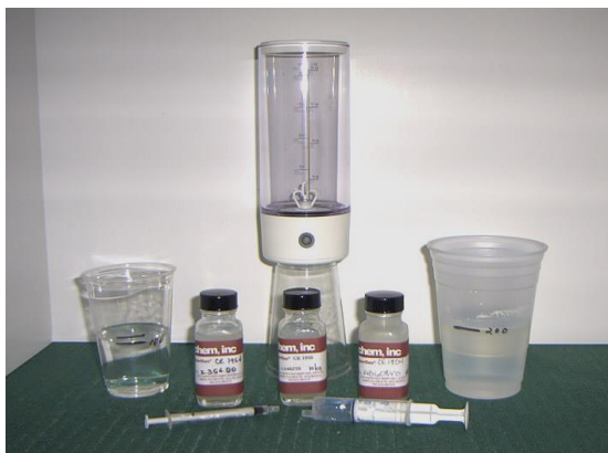
Figure 2. The Rapid Dewatering Test
