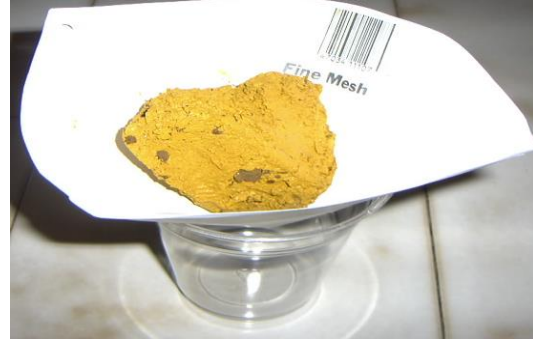
Figure 8. Filter cake- after 72 hours and passes paint filter test
