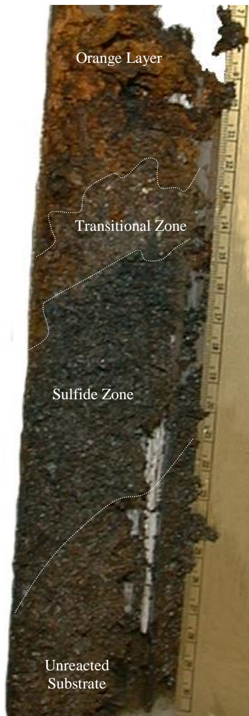
Figure 1. Photograph of a split sediment core from the LBOS showing the three mineralogical zones overlying unreacted substrate. Scale to the right is in centimeters.
