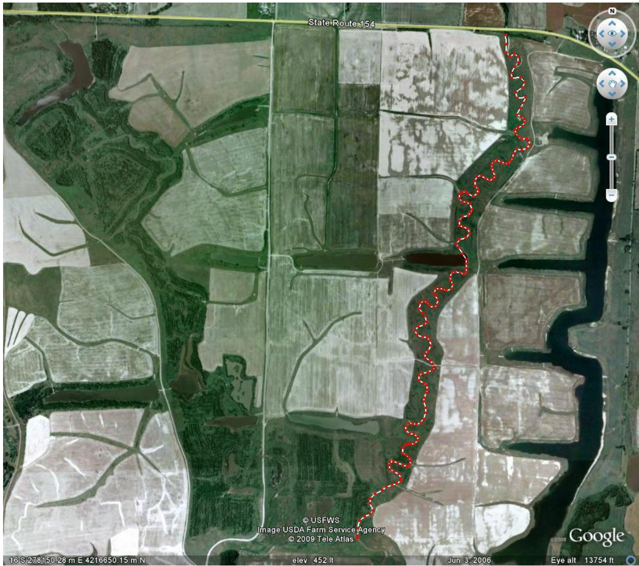
Figure 5. CONSOL Burning Star 4. Bonnie Creek 3.7- mile restoration relocated through reclaimed mine soils in the approximate pre-mine riparian corridor.
