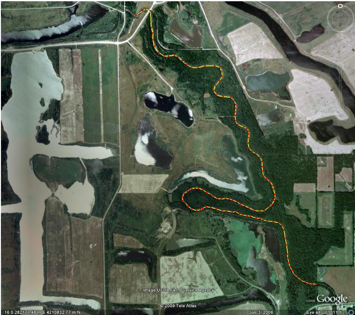
Figure 2. ARCH of Illinois Galum Creek restoration. Meander channel (4.3 miles) rerouted through unmined soils east of active mining area.
