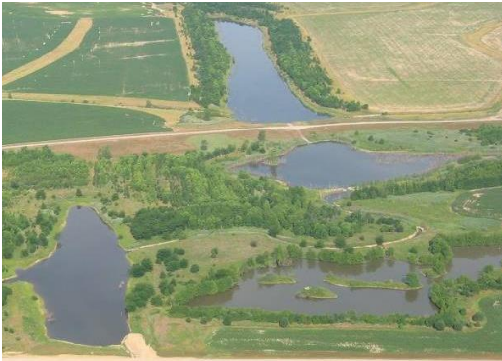
Figure1b. AFTER - CONSOL Burning Star 4 Mine. Galum Creek restoration incorporating diverse reclaimed land use (rowcrop, forest, wetlands) with channel relocation (Photo Date2005)
