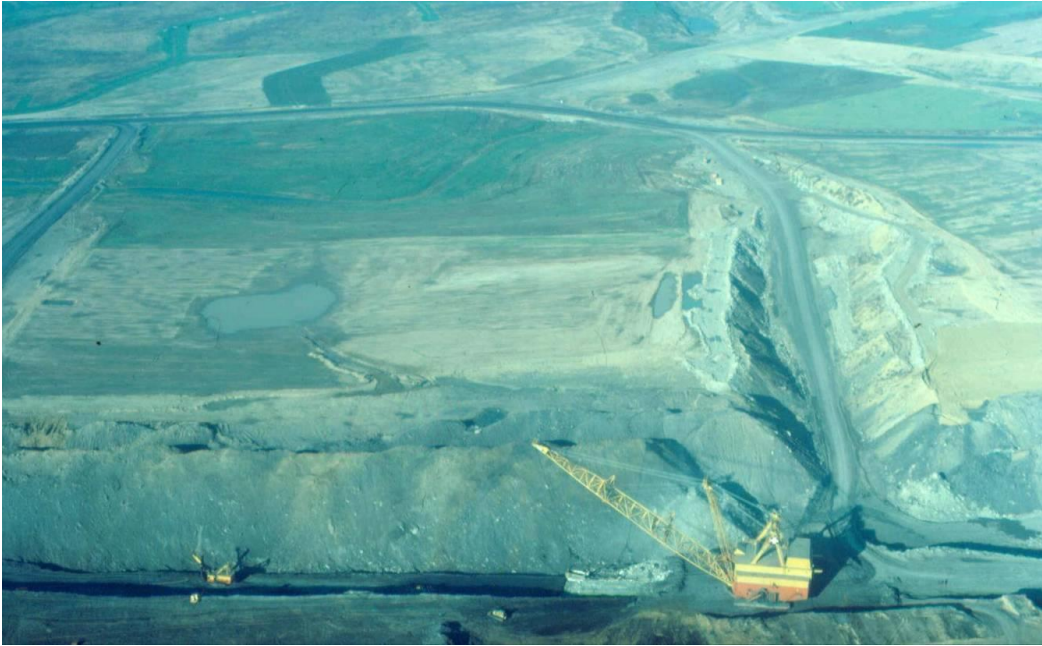
Figure1a. BEFORE - CONSOL Burning Star 4 Mine. Galum Creek restoration integrating meander channel construction with active mining. (Photo Date1985)
