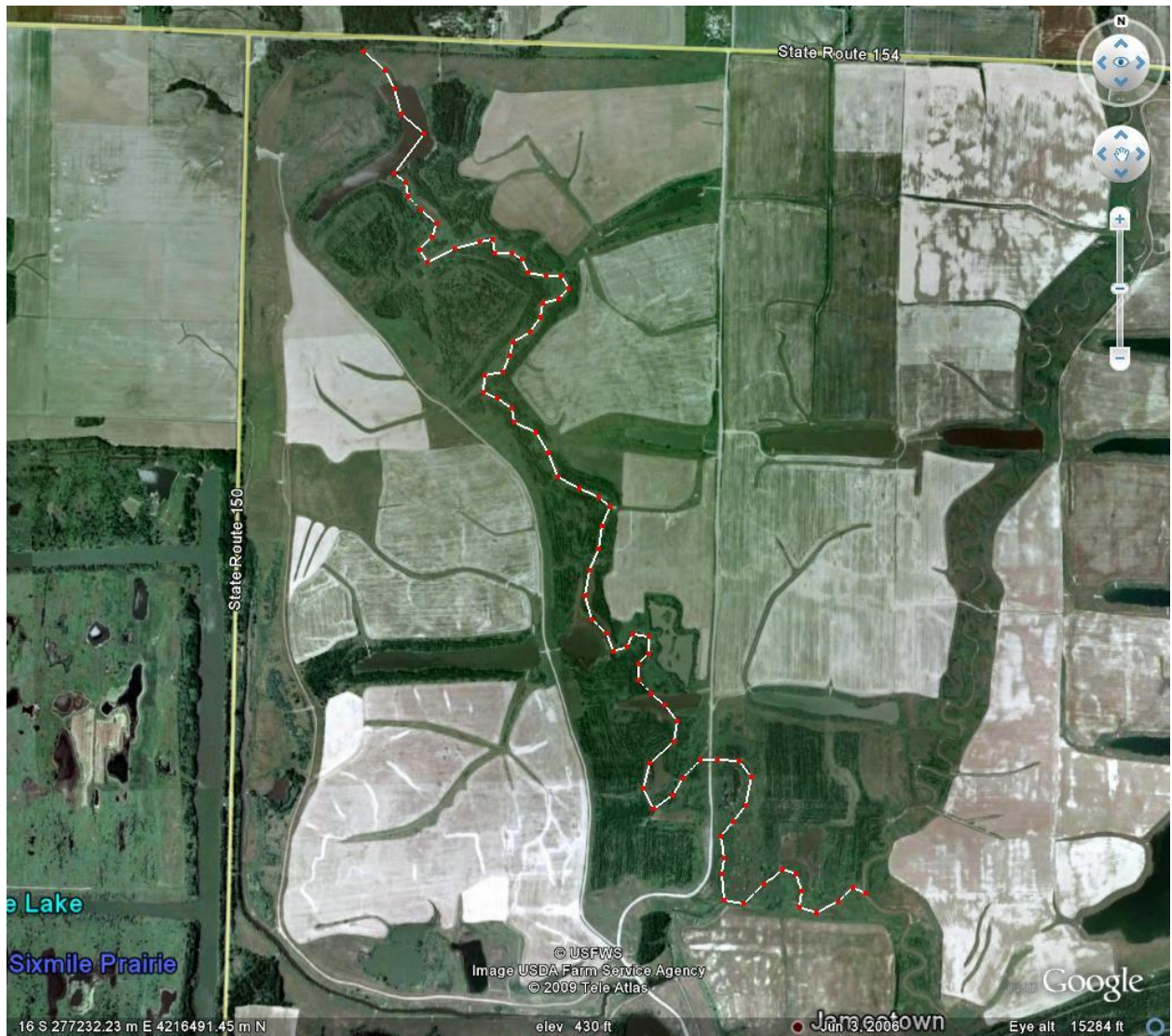
Figure 4. CONSOL Burning Star 4. Galum Creek 4.3- mile restoration relocated through reclaimed soils in the approximate pre-mine riparian corridor.
