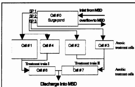
Figure 1. Schematic layout of the wetland demonstration system.
