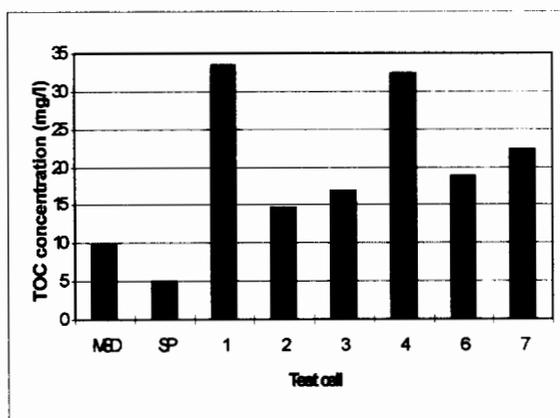
Figure 4. Change in total organic carbon (TOC) concentration due to the wetland treatment of MSD water. The plotted concentrations are averages of July and August.
