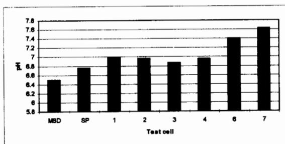
Figure 2. Increase in pH due to the wetland treatment of MSD water. The plotted pH values represent averages of July and August.
