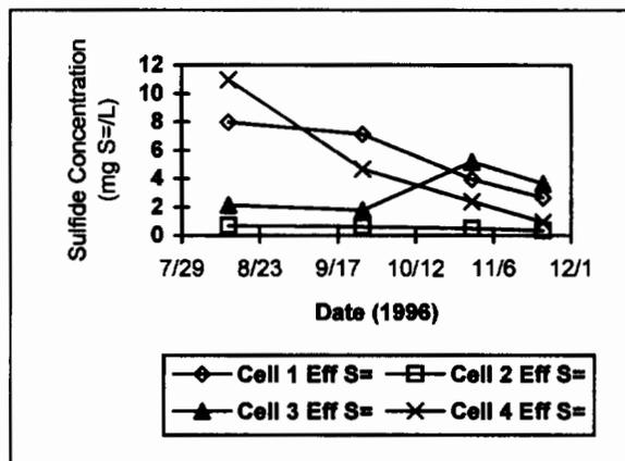
Figure 5. Sulfide concentration in the anoxic treatment cell effluents.
