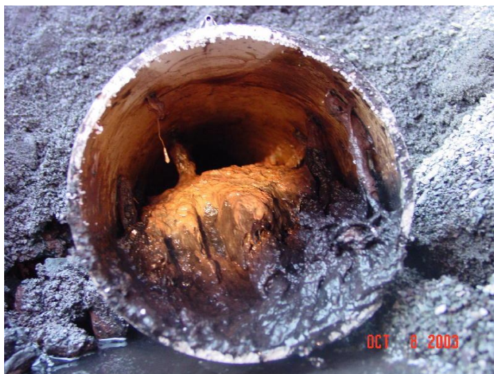
Figure 9. Biological growth in feed line to demonstration bed, October 2003
