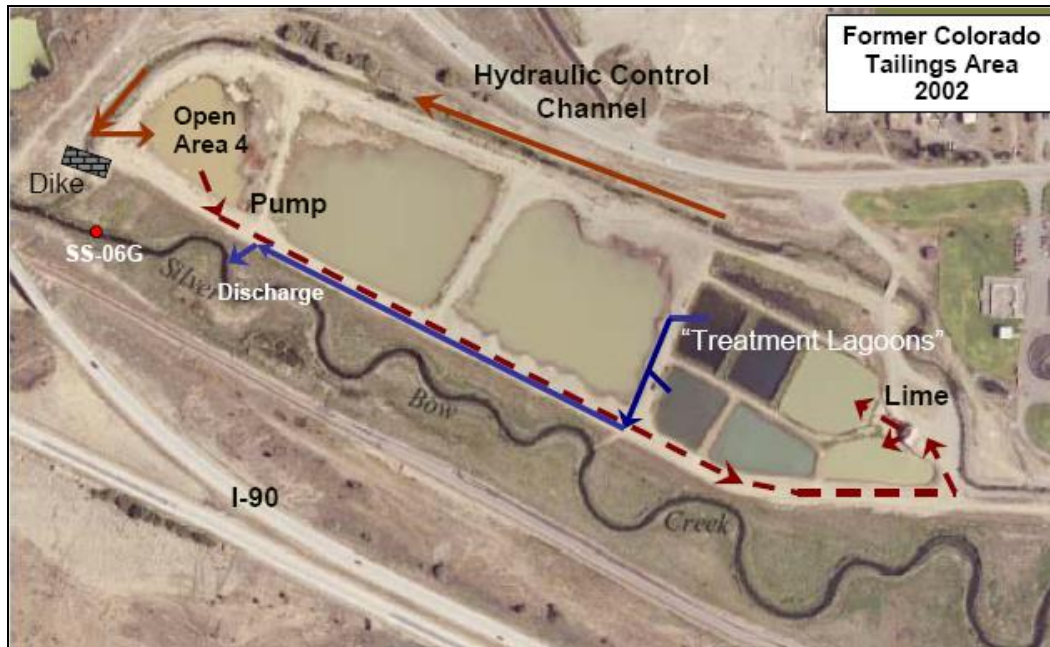
Figure 9. Aerial photograph showing routing of captured groundwater, treated water, and discharge to Silver Bow Creek.
