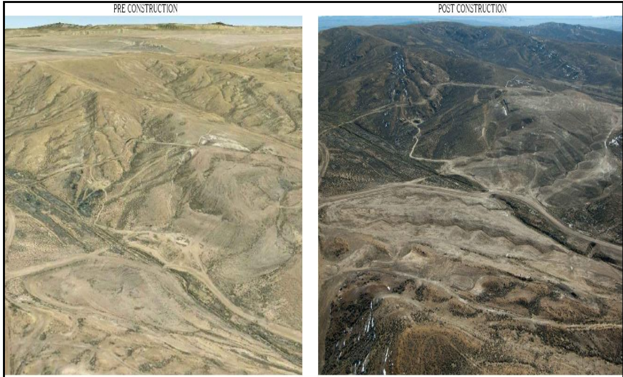
Figure 6. Lionkol Main Pits images before and after construction. The Main Pit was a “mountain top” mine, where the top of the hill was excavated and pushed over the sides.
